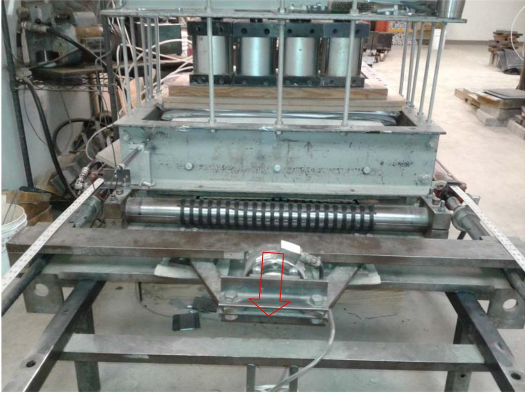
Figure A-4. Front view of the connection test setup.
