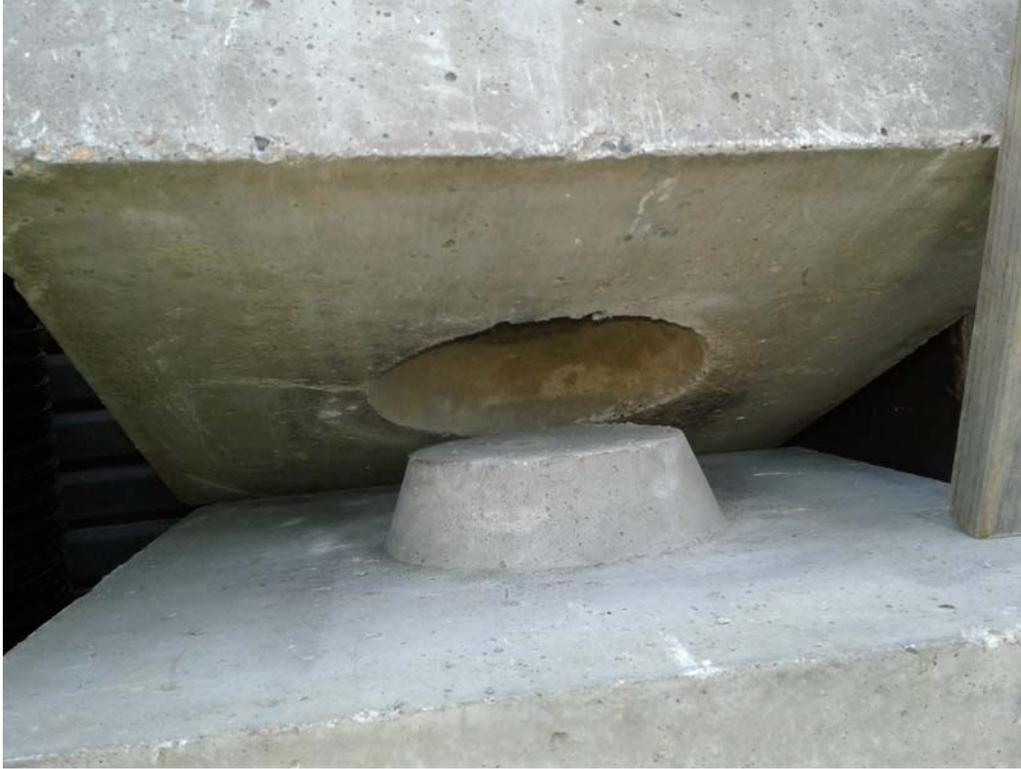
Figure A-2. Round cavity at the center of top block and knob at the center of bottom block.
