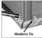
inches (8 inches for 8" Block) of each Trim Channel and place two prepared units on the Starter Ledges at each end of the corner. Because of the miter cuts, the ends should fit together snugly.
